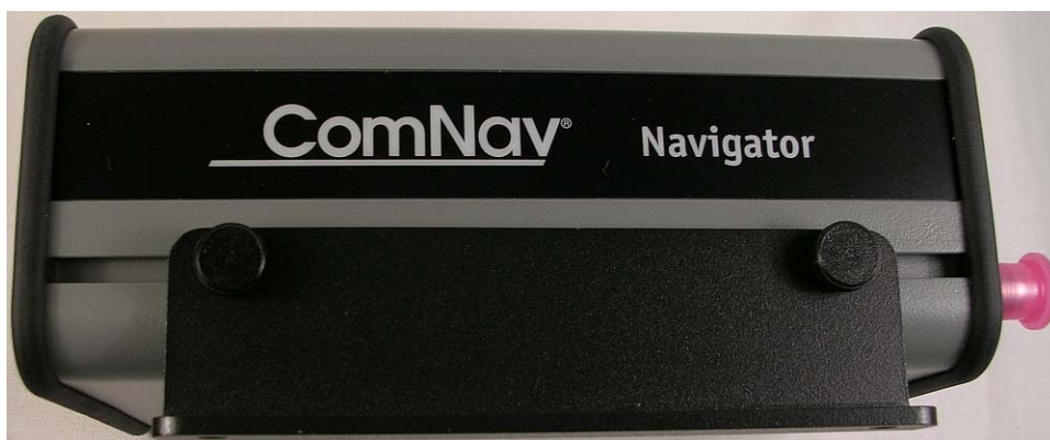
Figure 10 – Receiver Fastened to Bracket
